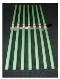
The MAGNUM® AD 2000 is a compact aeration unit based on the approved MAGNUM 2000 diffuser technology. The AD 2000 is a membrane diffuser for fine bubble aeration. It can be opperated continuously as well as in on/off mode.
