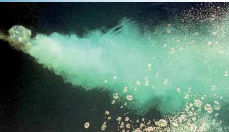
Fine bubble plume created by FUCHS spiral propeller
